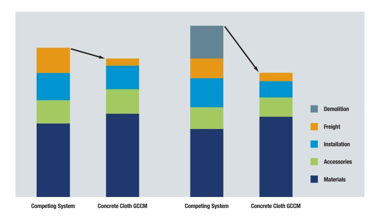
Concrete Cloth GCCM can lower total installed cost with less freight and faster installation.
